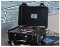
The STI-350 can also track and locate transponders designed to work with the receiver. These transponders allow divers to mark targets underwater and re-locate them up to 750 metres away. The STI-350 provides accurate range and bearing to the transponder to within 1m.
