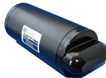
The VADR receiver's small size and rugged design allows for easy mounting on a ROV or AUV. Electronics and a highly directional hydrophone are contained in the pressure housing and are externally powered by the subsea vehicle through a 5-pin bulkhead connector. In addition, all telemetry data for controlling the VADR receivers and output data is accessed through this same connector.
