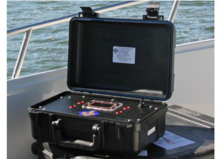
The STI-350 can also track and locate transponders designed to work with the receiver. These transponders allow divers to mark targets underwater and re-locate them up to 750 metres away. The STI-350 provides accurate range and bearing to the transponder to within 1m.
